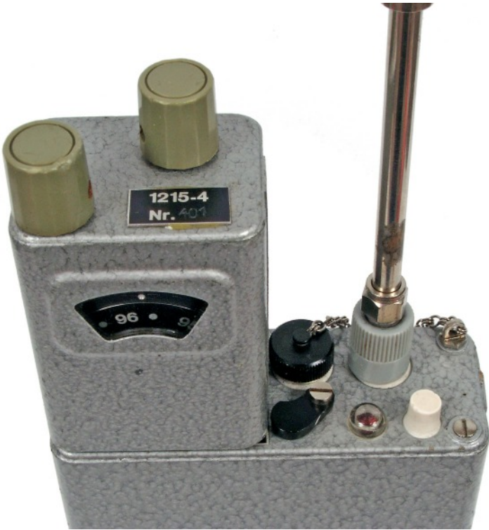
Top view of 31215-1 main receiver body and 31215-4 plug-in remote control unit. (above)
